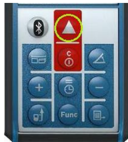
Fig. 19. Keypad of the rangefinder with a marked button that measures and simultaneously transfers the result to the program
